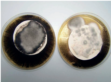
Testing of effectivity of film protection agents in coatings according to EN 15457
