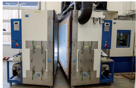
Differential climate testing of windows
