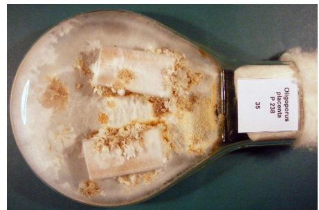
Fungus test of thermally modified timber (TMT)
