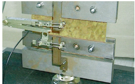
Determination of the locking strength of Floorings
