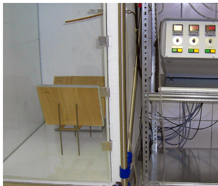
Determination of the formaldehyde emission
