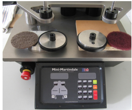
Test device for polishing resistance acc. to IHD-W-475
