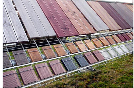
Weathering of samples
