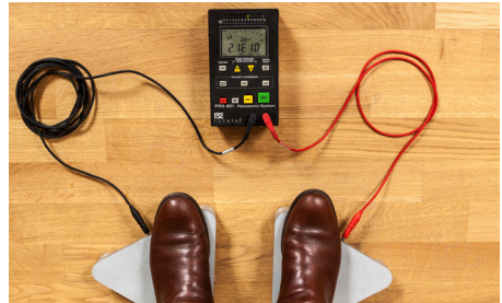
Determination of the electrical resistance acc. to EN 1081
