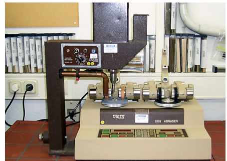
Determination of the abrasion resistance with Taber Abraser with integrated Grit Feeder (falling sand-method)
