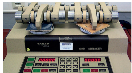
Determination of abrasion resistance
