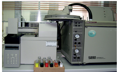
Determination of VOC-content by Headspace GC/FID
