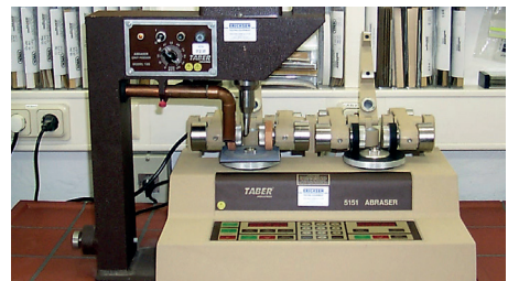
Determination of the abrasion resistance with Taber Abraser with integrated Grit Feeder (falling sand-method)
