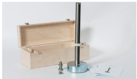
Determination of impact resistance acc. to EN 17368 for laminate floor coverings
