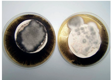
Testing of effectivity of film protection agents in coatings according to EN 15457
