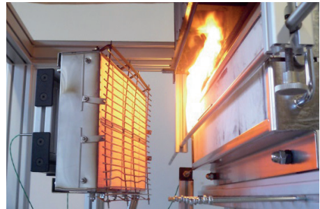
Testing acc. to FTP Code 2010 for determining surface flammability (interior maritime use)
