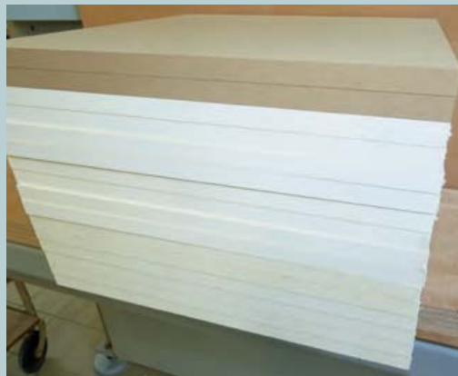
Abb. 2: Hergestellte MDF aus Altpapier (Referenz Kiefer) Fig. 2: MDF made from waste paper (pine as a reference)
