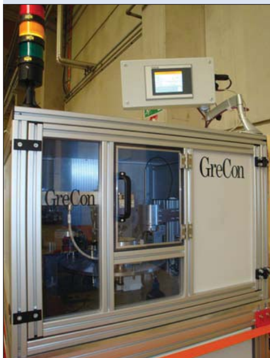
Fig. 1: Apparatus for determining formaldehyde emissions from wood-based chips
