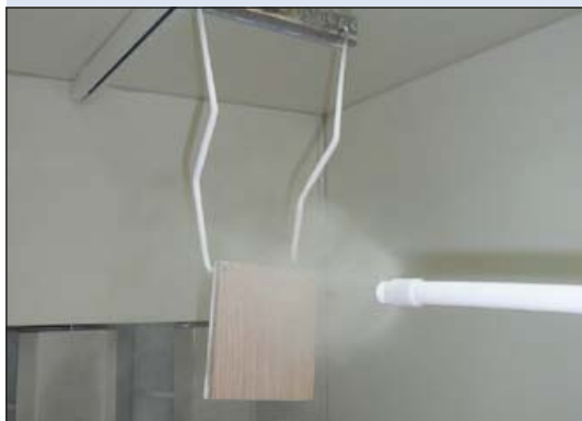
Fig. 1: Use of a Tribo spray gun for applying powder to veneered samples
