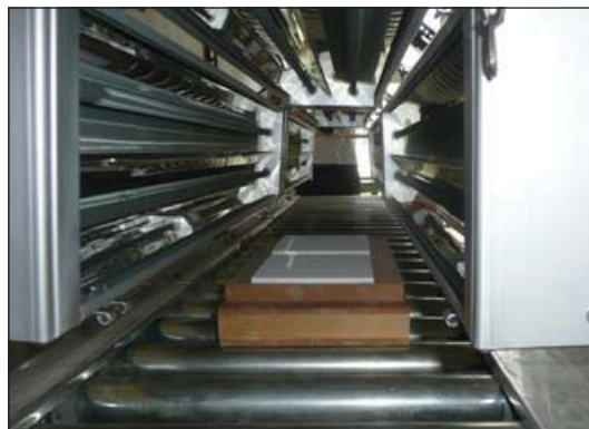
Fig. 2: Ceramic-coated IR radiators at IHD's technical laboratory melting the powder lacquer applied to veneer
