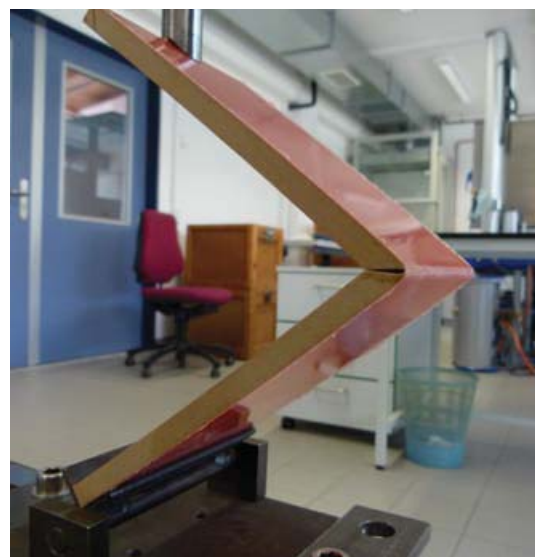
Fig. 1: Pressure test on a corner element
