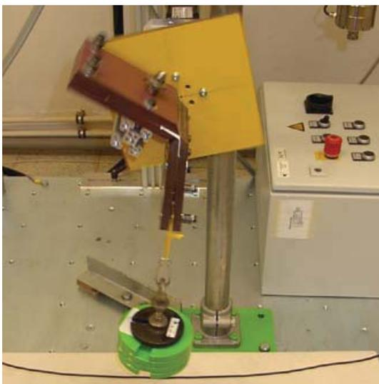
Fig. 2: Tumble test with an additional weight
