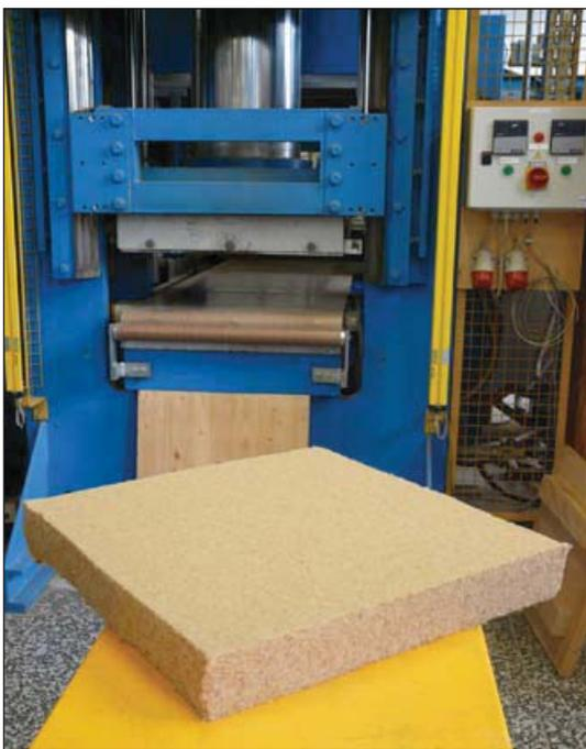
Fig. 1: Insulating wood-fibre board of chemically modified fibres
