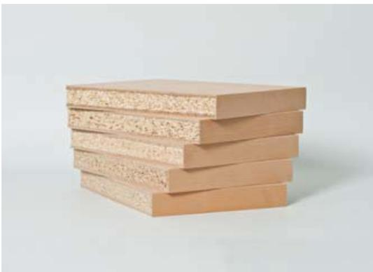
Fig. 2: Coated chipboard samples with chip mixes of chips from cutting and chipping (spruce), density  $480 \text{ kg/m}^3$ , with polystyrene (top), cork (second from top), without filler material (middle) compared to a chipboard of industrial middle-layer chips without filler material of a board density of  $480 \text{ kg/m}^3$  (second from bottom) and  $600 \text{ kg/m}^3$  (bottom)
