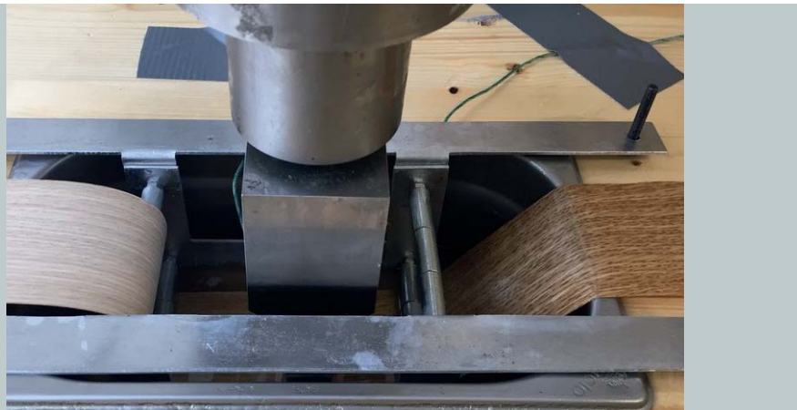
Abb. 1: Kontinuierliche Furnierimprägnierung mittels Leistungultraschall Fig. 1: Continuous veneer impregnation by means of power ultrasound
